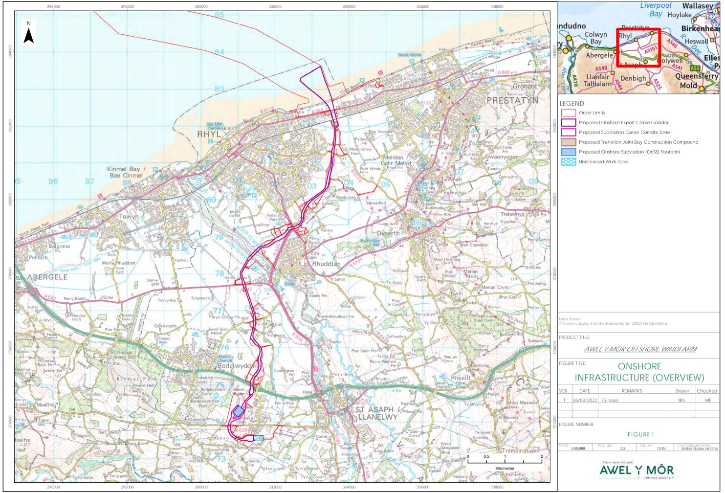
The transmission voltage will be up to 400 kV, and the onshore ECC will be approximately 12 km in length from the TJBsto the existing National Grid Bodelwyddan substation.
